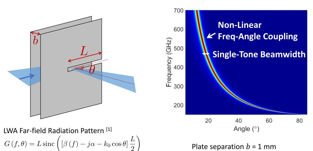
Plate separation b = 1 mmSlot length L = 3 cm
