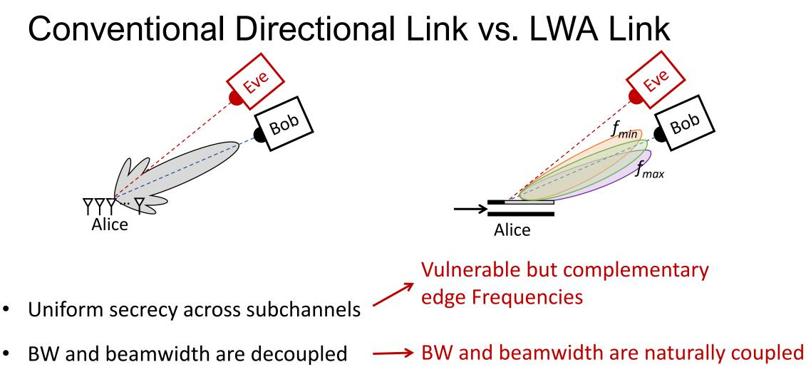
• A wider beam is less secure
